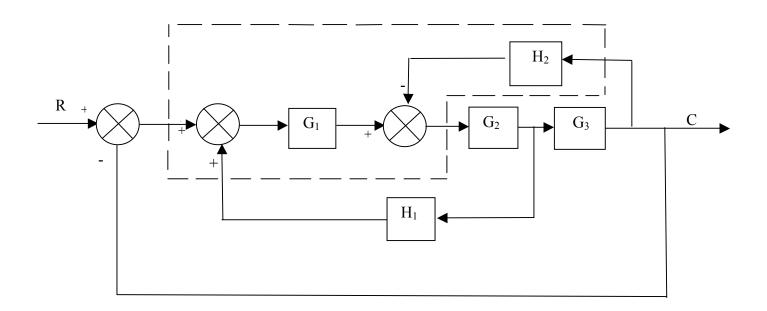
In this case, we will manipulate the feedback loop containing  $H_2$  to be outside the loop containing  $H_1$ . Then moving the summing junction before  $G_1$ , the highlighted area (indicated by dotted line) may be written:
